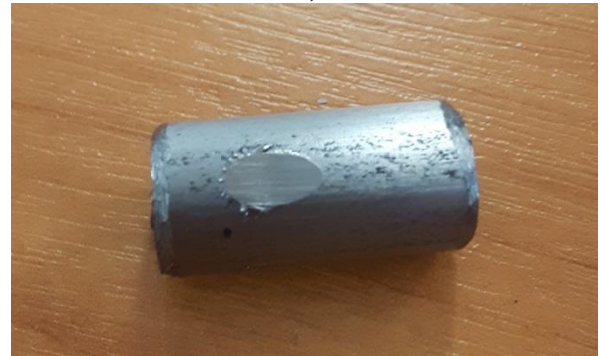
Fig. 3. Timken sample after 7 minutes of abrasion
