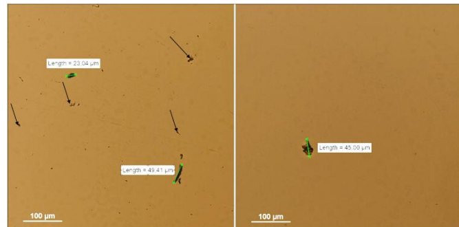
Fig. 7. Sample No. 1 after mileage of 49000 km
